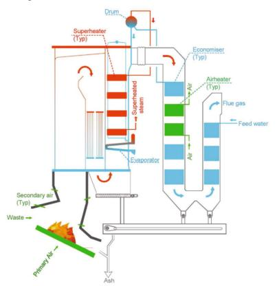
TYPICAL VERTICAL ARRANGEMENT WASTE TO ENERGY BOILER
